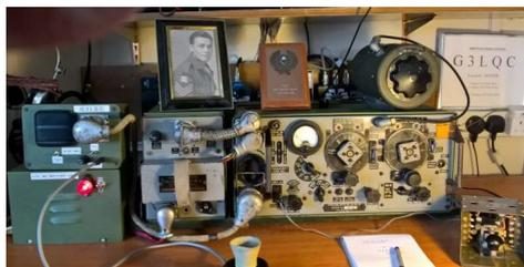
The equipment runs in 3 bands: 220-270 MHz 'B' Set, 2.- 4.8 MHz and 4.8 - 8.0 MHz. 'A' set. I have worked one Russian station on CW with this equipment who gave me 599. I think he was being kind as the CW note of the 19 set sounds like a chirping canary and so I should have got 599c. In the old days, (50s), you were lucky if your homebrew didn't have a chirpy 'c' note.
